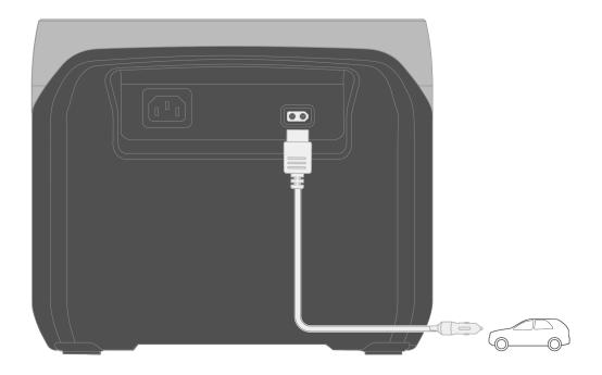
You can recharge the product through the car power outlet. The product supports 12V/24V car chargers and a maximum charging current of 8A. EcoFlow takes no responsibility for any loss or damage caused by failure to follow instructions.
