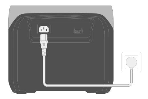
Please use the AC charging cable included in the package and plug the cable directly into a wall outlet instead of an extension socket.
